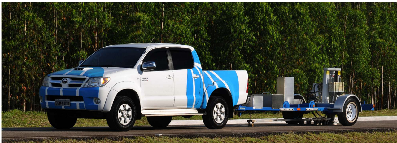
Figura 2 – Vista do Falling Weight Deflectometer Dynatest 8000.
